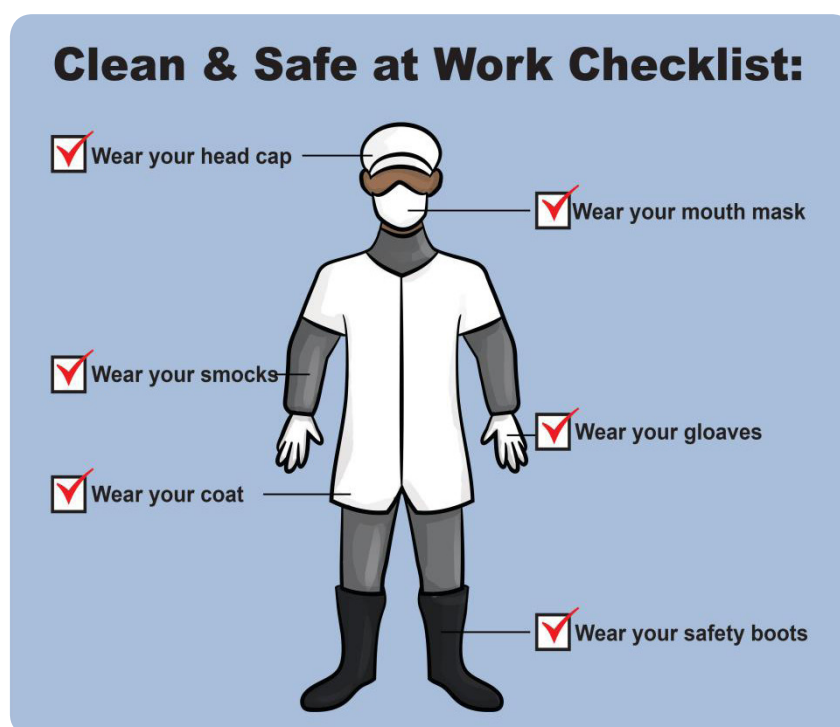
Figure 133: Recommended PPEs for applying pesticides
