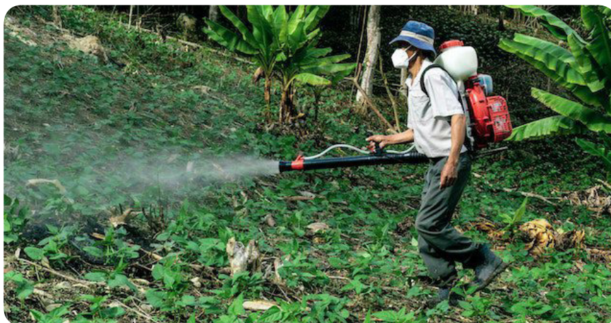
Figure 84: Spraying using a mechanical knapsack sprayer
