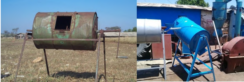
Figure 91. Drum mixers locally fabricated at a welding shop
